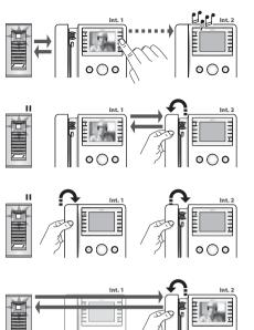
When an active call is open, select the internal receiver to which the call is to be transferred.
